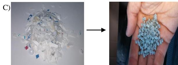
**Figure 2.** Images of input consisting of a) Polyethylene (PE) and ultra-high molecular weight PE (UHMWPE), b) post-consumer recycled (PCR) laminated film, c) Polyvinyl chloride (PVC) mixed waste and the final product.
