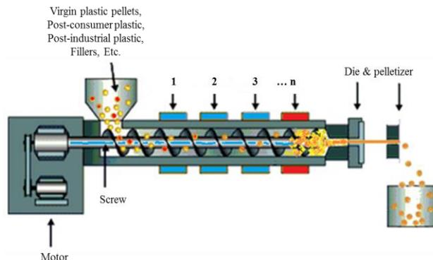
**Figure 1.** Schematic of SSSP apparatus
